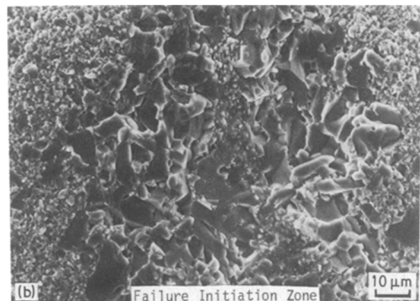
Figure 11 SEM fractographs showing failure initiation at an “agglomerate” of large-grained alumina grains.
