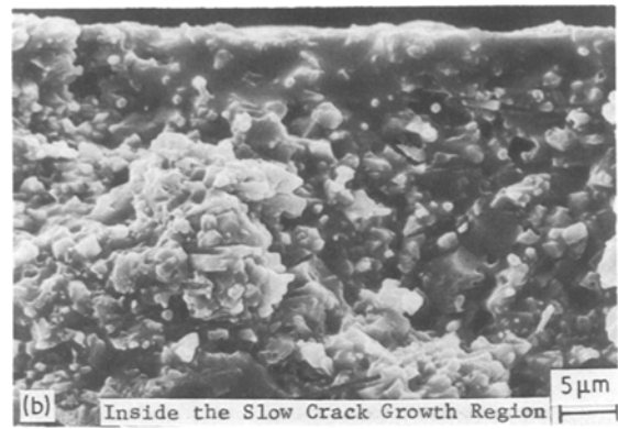
Figure 14 Typical fracture surface as seen in SEM for a specimen tested in stress rupture mode.
