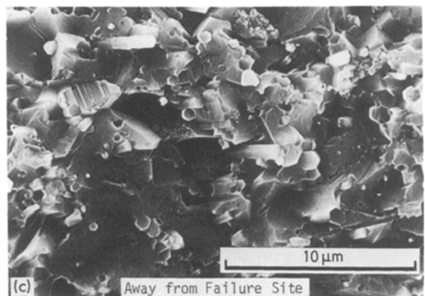
Figure 4 Typical failure site seen in SEM for an alumina composite specimen tested in fast fracture mode.
