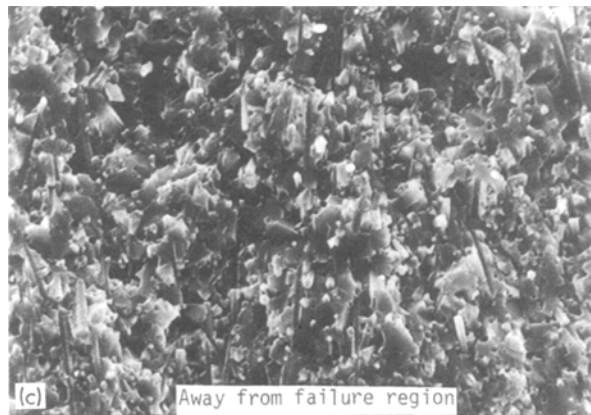
Figure 6 SEM fractographs showing failure initiation at a sub-surface flaw.
